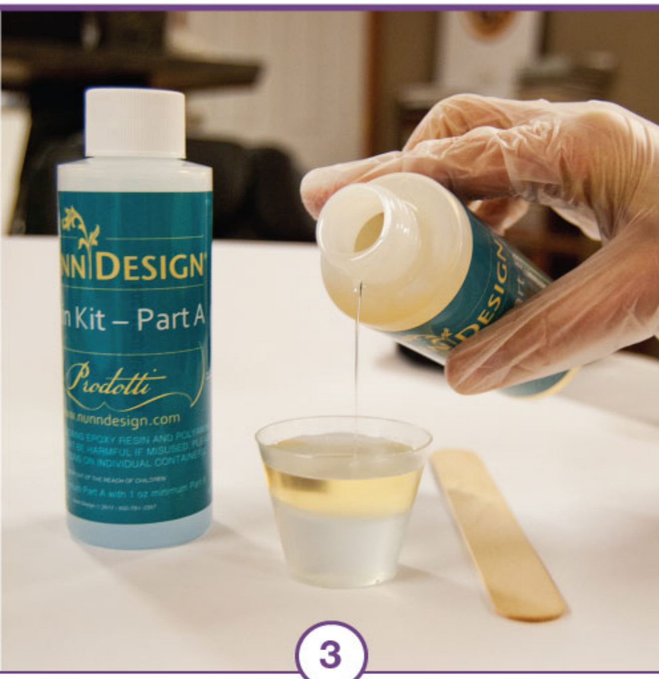
Pour equal parts of A, then B, of Nunn Design 2-Part Resin into cup, mix for 2 minutes and put under lamp for 5 min.
