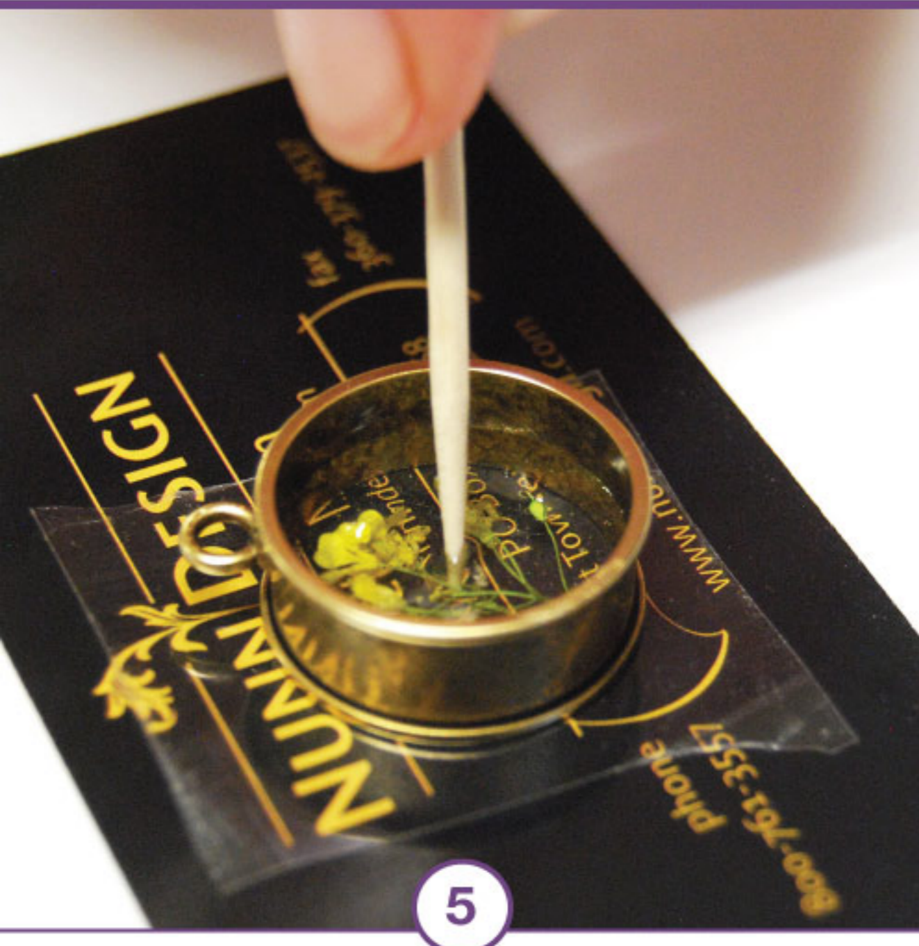
Use a toothpick to agitate the resin and make sure there aren't any air bubbles.
