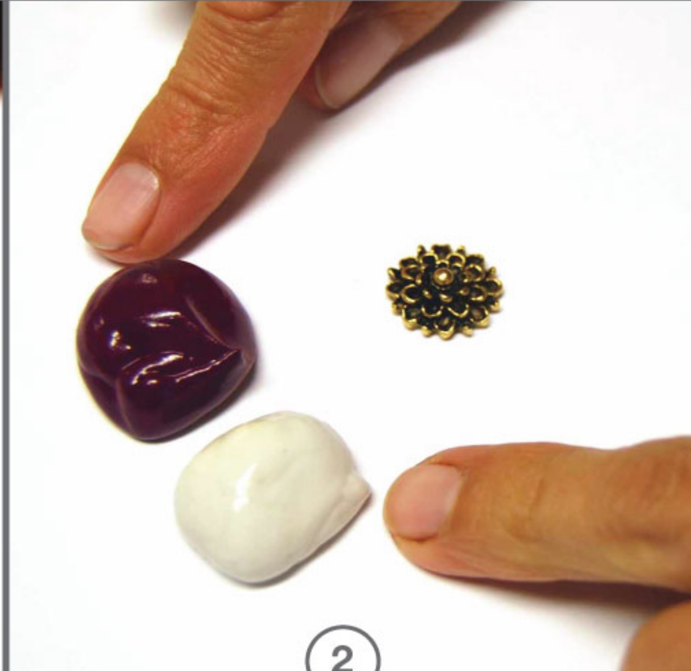
2 Use equal sized balls Part A and B of Silicone Putty. Be sure the balls are large enough to allow the impression of the charm.
