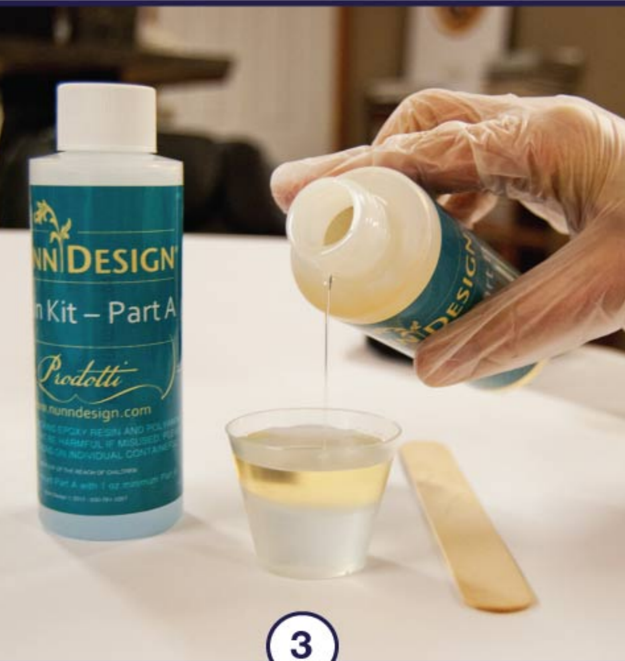
3 Pour equal parts of A, then B, of Nunn Design 2-Part Resin into cup, mix for 2 minutes and put under lamp for 5 min.
